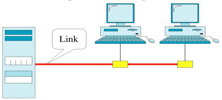
A multipoint (also called Multidrop) connection is one in which more than two specific devices share a single link.
