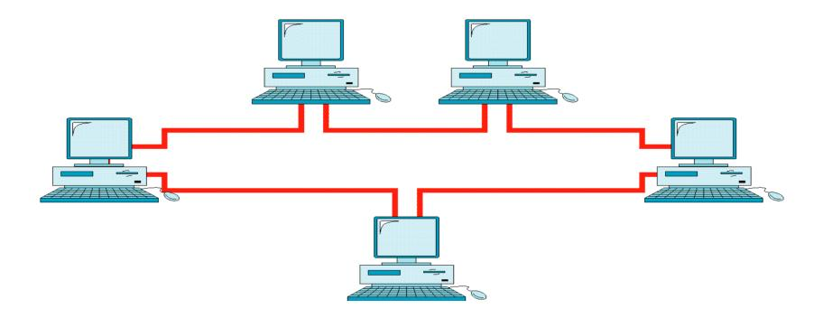
In a ring topology each device has a dedicated P2P connection with only the two devices on either side of it.
